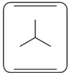
**Baking/roasting with heating from the bottom and the top** - with air thermo-circulation switched on in the interior of oven.
