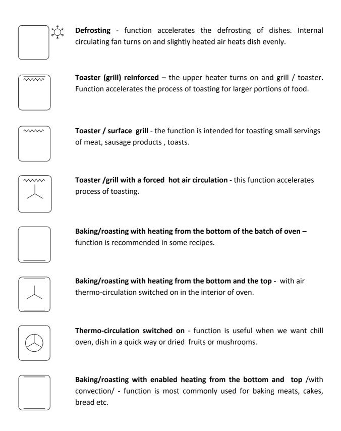
Description of the symbols in the "B" section of the control panel - Setting the clocks
